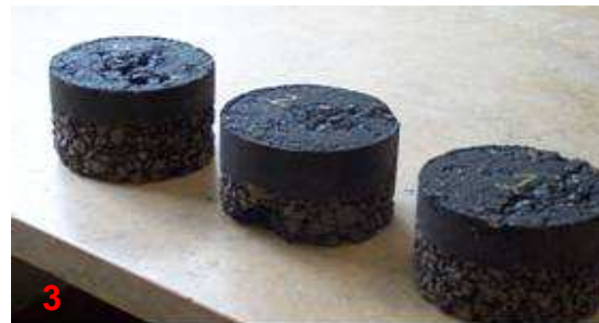
3. Samples after soaking in fuel
