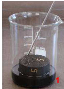
1. Test samples parcialy soaked in fuel
