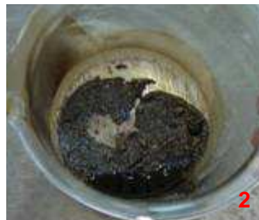
1. Test samples parcialy soaked in fuel
